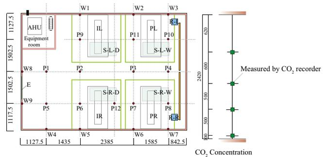
Fig. 6 Measurement points of experimental room [mm]
