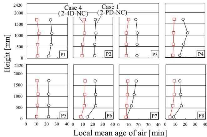
Fig. 10 Local mean age of air (contaminant source position:PD and 4D, without curtain, air change rate: 2 times·h<sup>-1</sup>)
