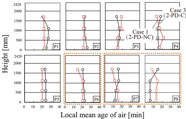
Fig. 9 Local mean age of air (contaminant source position:PD, with and without curtain, air change rate: 2 times·h<sup>-1</sup>)
