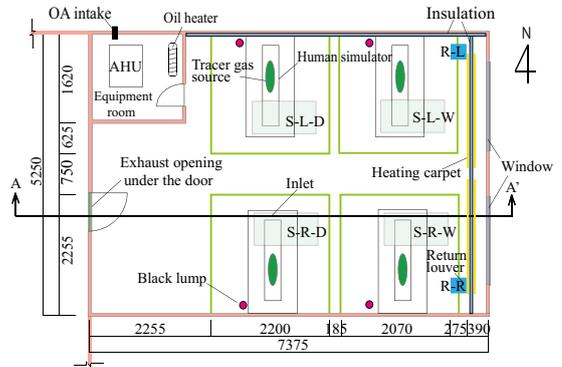
Fig. 4 Plan of experimental room [mm]
