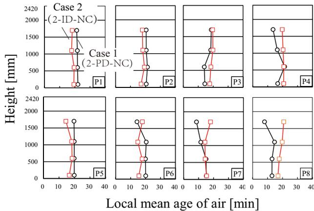
Fig. 8 Local mean age of air (contaminant source position:PD and ID, without curtain, air change rate: 2 times·h<sup>-1</sup>)
