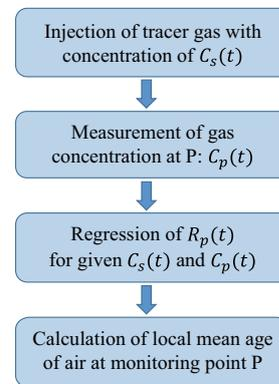
Fig. 2 Calculating flow chart of local mean age of air
