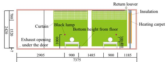
Fig. 5 A-A' section of experimental room [mm]
