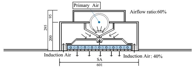
Fig. 3 Air-conditioning system with induction panel
