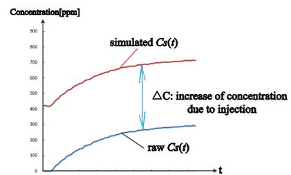
b) Injected tracer gas from supply
