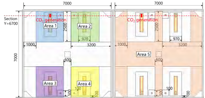
Fig.7 Location of the temperature data's pick up area
