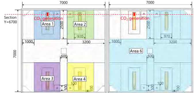
Fig.8 Location of the concentration data's pick up area
